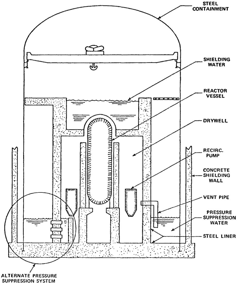
**Fig. 56.10** Mark III containment for BWR. (Used by permission of Pergamon Press, Inc., New York.)
