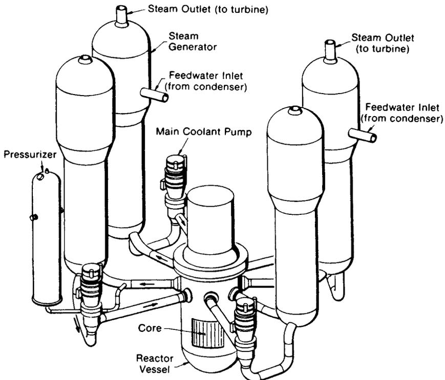
Fig. 56.8 Typical arrangement of PWR primary system.
