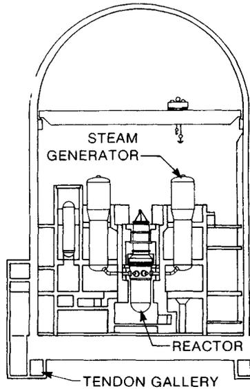
Fig. 56.9 Typical large dry PWR containment.
