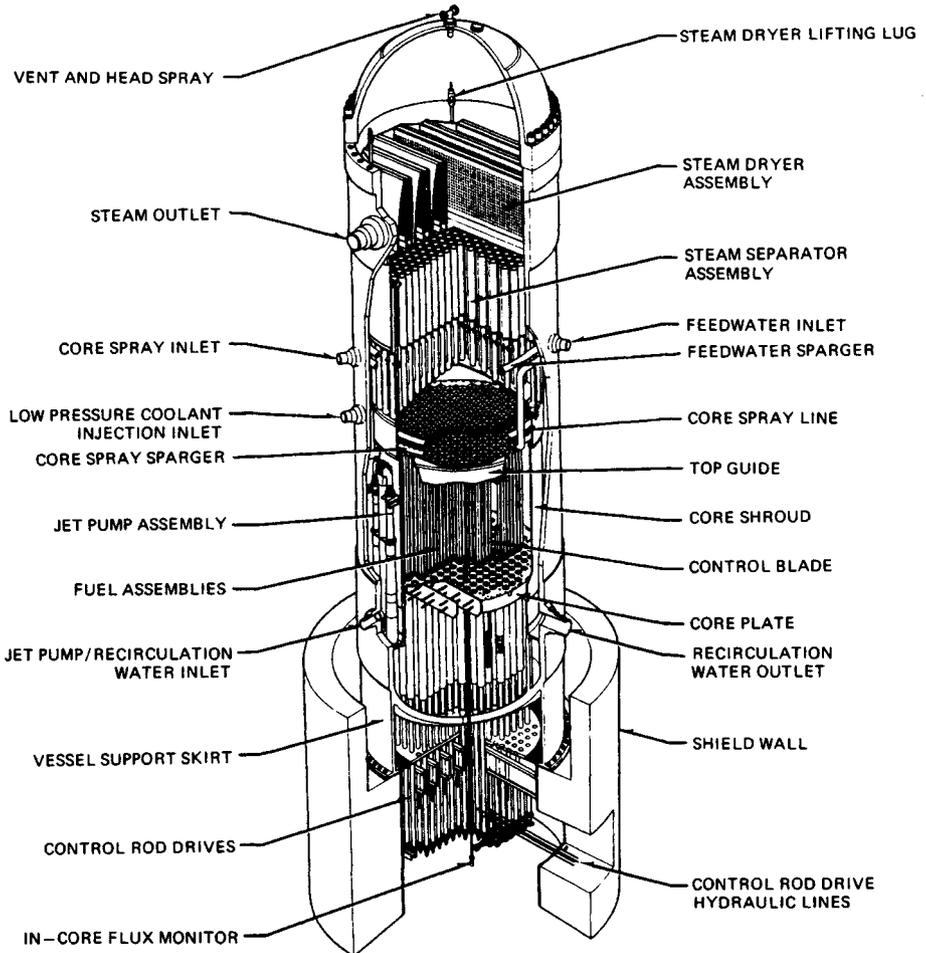
Fig. 56.3 Typical BWR vessel and core configuration. (Courtesy General Electric.)
