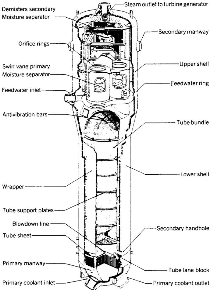
**Fig. 56.2** Typical PWR steam generator.
