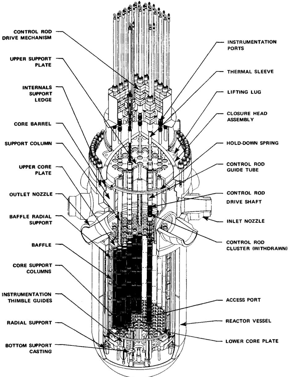
Fig. 56.1 Typical vessel and core configuration for PWR. (Courtesy Westinghouse.)
