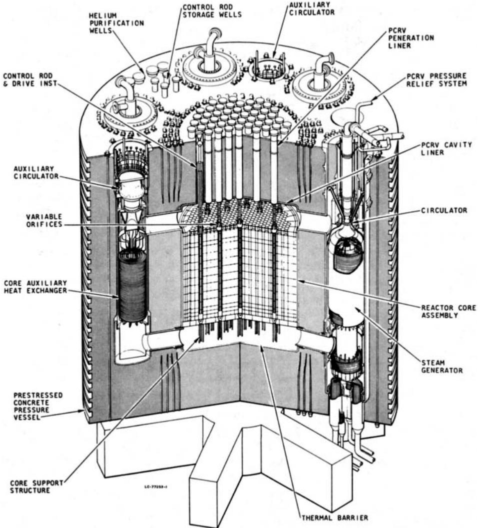
Fig. 56.5 HTGR pressure vessel and core arrangement. (Used by permission of Marcel Dekker, Inc., New York.)
